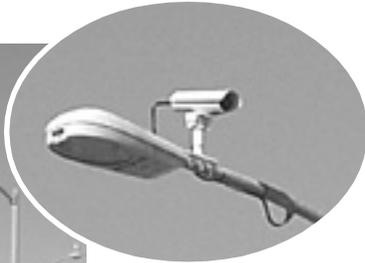
**Video detection** is proving to be very accurate for detecting bicycles. The intersection is separated into zones of detection that include each lane
